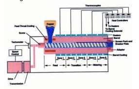
In some cases a screen pack and breaker plate are positioned at the end of the barrel to filter out foreign contaminants that may have entered the hopper. The screen pack also increases backpressure in the barrel, contributing to a homogenous melt and steady flow. The breaker plate holds the screens, gives them support and contributes to the backpressure.
